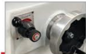
Hidrolik tabla hız ayar kolu (X Eksen) Hydraulic table speed adjustment arm (X axis)
