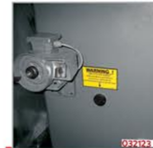
Çakı bileme motoru (Opsiyonel) Diamond (tool) dresser (to sharpen the chip braker) (Optional)
