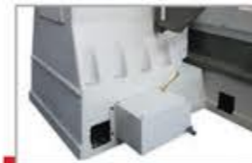
Atık yağ tahliye deposu Waste oil release storage
