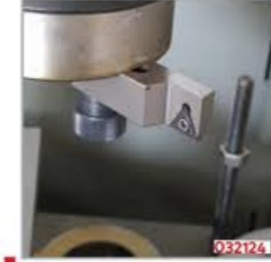
Fatura kalemi (Opsiyonel) Boring tool component with a dead-end hole tool (Optional)
