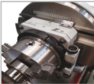
Yatay gezinti strok cetveli Horizontal movement strock indicator
