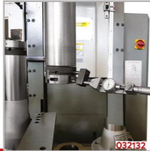
Paso mikrometresi (Opsiyonel) Feed dial gauge micrometer (Optional)
