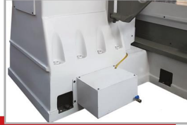
Atık yağ tahliye deposu Waste oil release storage
