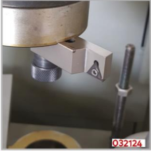
Fatura kalemi (Opsiyonel) Boring tool component with a dead-end hole tool(Optional)
