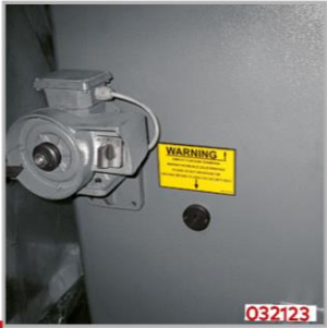
Çakı bileme motoru (Opsiyonel) Diamond (tool) dresser (to sharpen the chip braker) (Optional)
