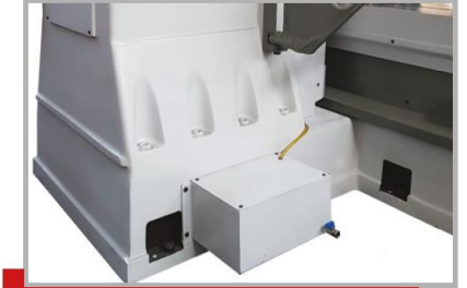
Atık yağ tahliye deposu Waste oil release storage
